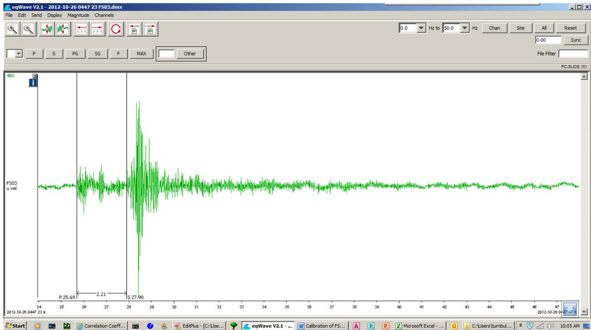
Figure 22: Earthquake recorded on FS03 on 26 October 2012
